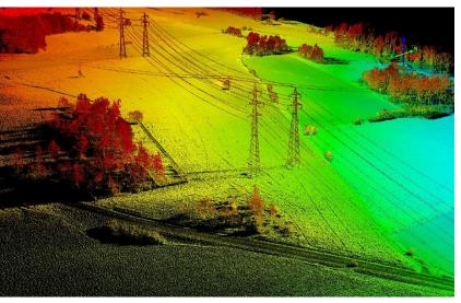
Working with an industry-leading LiDAR and imagery collection partner, Lux Modus classified 873 km of transmission powerlines. Completed in stages, this project required detailed classification and quality control.
